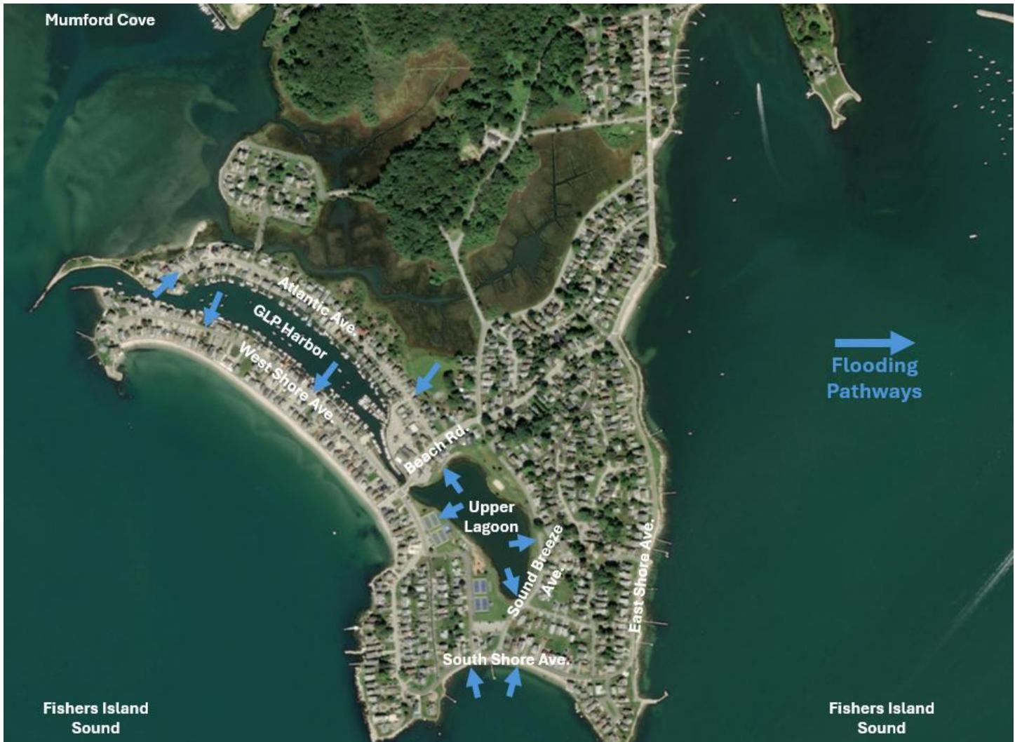
Figure 12: Flooding Pathways at Lower Stillwater Elevations - During Large Tides and 1-2 Year Storm Events
