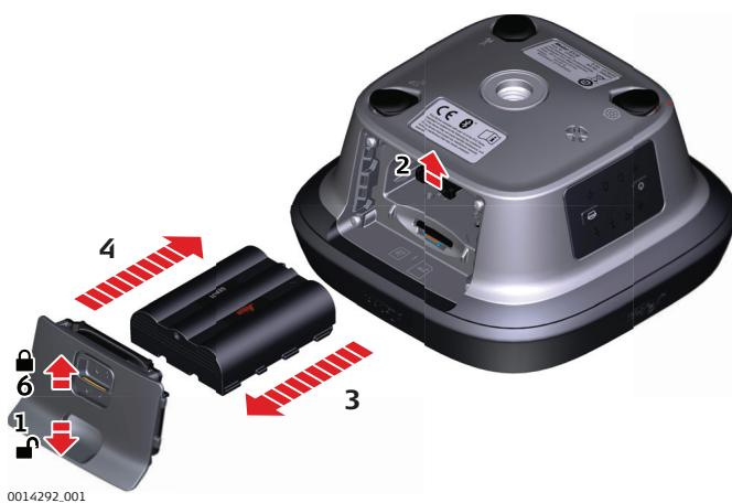
1. Push the slide fastener of the battery compartment in the direction of the arrow with the open-lock symbol. Remove the cover.
